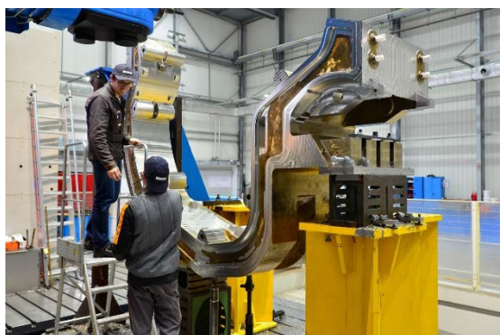
Figure 8: Divertor Cassette Body prototype in the last stages of completion
